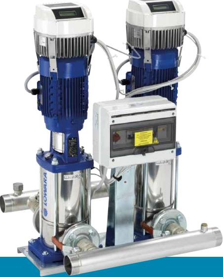
HYDROVAR® is a pump or wall-mounted variable speed microprocessor based system controller, and was the world's first of its type to manage motor speed and match pump performance to a range of hot and cold water applications. Due to the unique modular design the HYDROVAR® unit can be mounted or retrofitted to any existing centrifugal pump which has a standard IEC motor.
